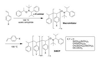
Scheme 1. Synthesis of macroinitiators and SiBCPs by LFRP at 100 °C.
