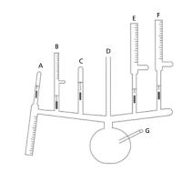
Figure 2. General set-up for a glass polymerization reactor.
