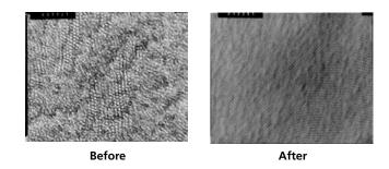
**Figure 1.** Transmission electron micrograph (TEM) images of  $PAcOSt-PSi_2St$  (21/79 v/V) before and after  $O_2$  plasma for 10 minutes, showing intact cylindrical morphology.
