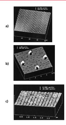
**Figure 2.** AFM images of a) 250nm punctures in ca. 100 nm thick film of fluoroalkyl-substituted HBFP; b) expelled material adjacent to punctures; c) imprint of 50–60 nm thick lines spaced 210 nm apart. Imprinting: Krchnavek, Dept. of Electrical Engineering, Washington University, St. Louis; AFM: Tomasz Kowalewski, Dept. of Chemistry, Carnegie Mellon University.
