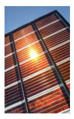
Dye solar cells (DSCs) are third generation solar cells with the promise of high efficiency combined with low production costs. While present day DSCs provide light-to-electricity conversion of up to 11%, significant further improvement is envisaged through optimized materials and novel cell and module architectures.
