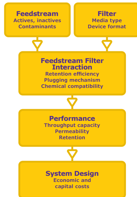
Figure 1: Considerations for assessing filter performance
