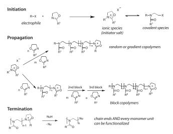
Figure 1. General reaction scheme of the living ring-opening polymerization of 2-oxazolines.
