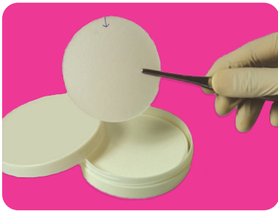
Fig 1. A membrane is taken from the box under aseptic conditions. Once removed, it can be marked (arrow) for easier later alignment of the colony patterns on the plate and the membrane.
