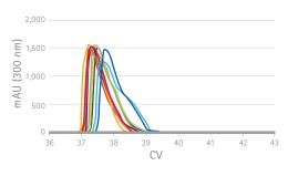
A. Eshmuno® A resin elution peak profiles with different citric acid elution conditions
