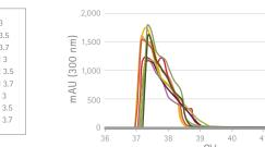
B. Eshmuno® A resin elution peak profiles with different acetic acid elution conditions
