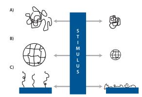
Figure 2. Classification of stimuli-responsive polymers by their physical form and their response to external stimuli. A) Linear free chains in solution will undergo a reversible collapse after stimulus is applied. B) Covalently crosslinked reversible gels where swelling or shrinking of the gels can be triggered by environmental change. C) Chain adsorbed or surface-grafted form, where the polymer reversibly swells or collapses on the surface once an external parameter is changed.<sup>11</sup>
