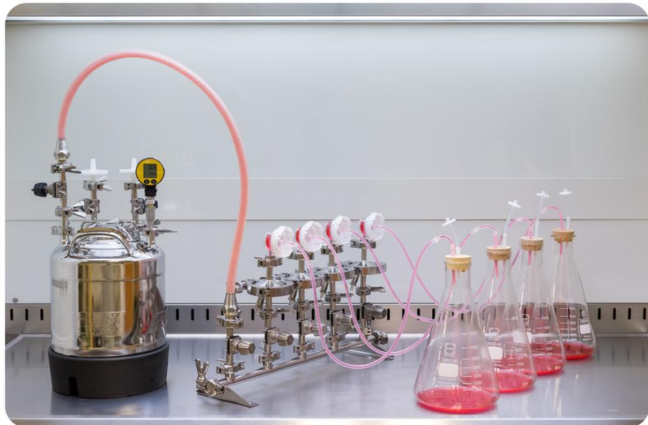
Figure 1. Small scale filter test set-up.
