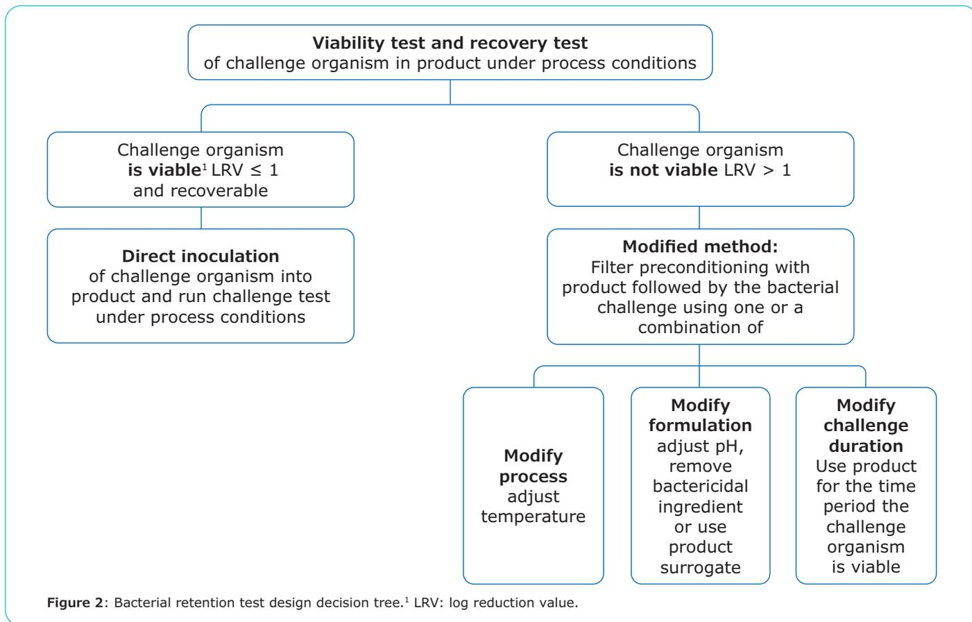
Figure 2: Bacterial retention test design decision tree.<sup>1</sup> LRV: log reduction value.
