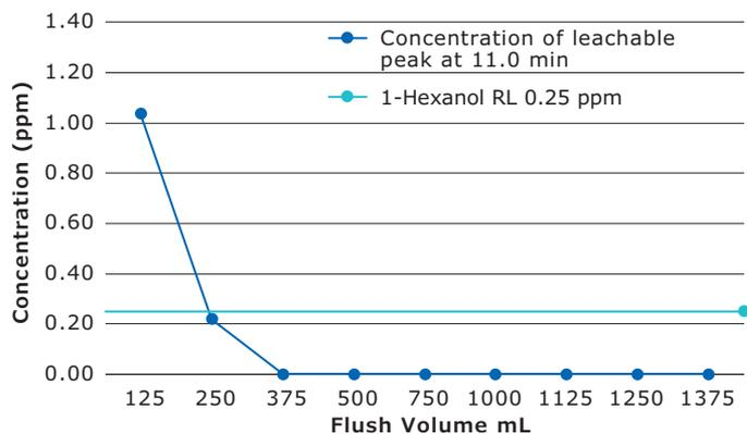
**Figure 5:** Examples of initial volume discarding for leachable peak at 11.0 min from 4" Durapore® 0.22 µm Gamma Irradiated filter.
