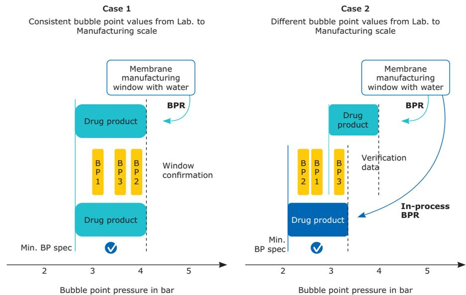
**Figure 7:** In-process monitoring of FIT limits. Case 1: production scale confirmation of small-scale results. Case 2: some production scale values fall outside small-scale limits prompting in-process determination of FIT limits.
