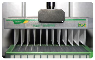
Figure 2. Supel™ BioSPME 96-Pin device maneuvered by automated liquid handing system gripper.
