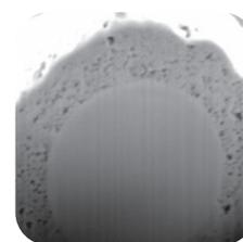
Chromolith® HPLC columns are based on a unique monolithic architecture that is resistant to matrix components due to large macropores in the silica skeleton. The large molecule version, Chromolith® WP, is compatible for biomolecules as the mesopores are 300 Å in diameter.
