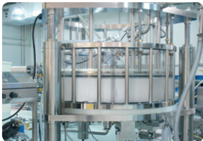
Large-scale column (1.6 m) packed with ProSep® media.
