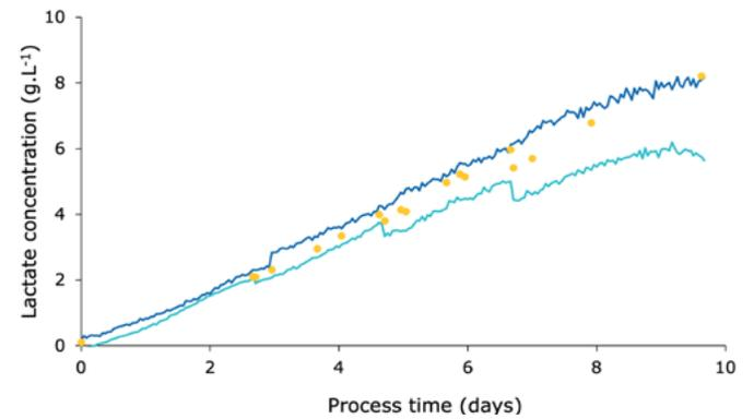
**Figure 3:** In-line real-time monitoring comparison of the standard methodology (light blue line —) vs the synthetic models methodology (dark blue —) with regards to off-line reference measurement (yellow dots ●)
