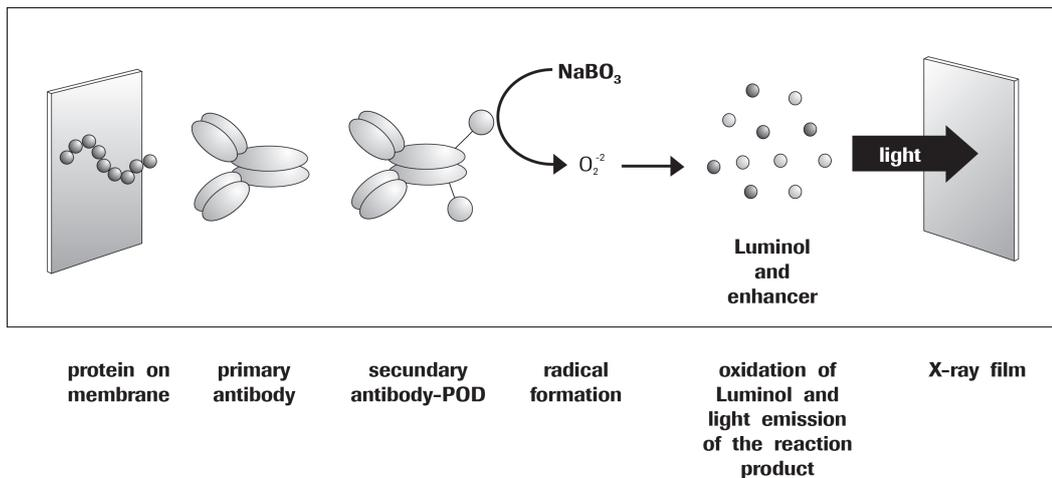
**Fig. 2:** Protein detection principle.
