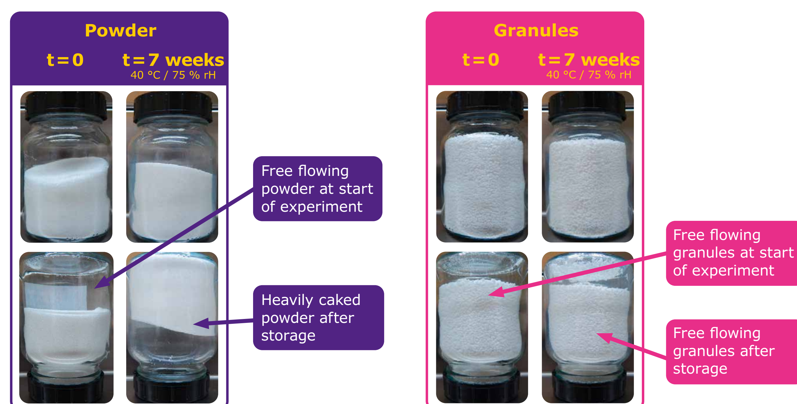
Figure 3: Comparison of caking behavior of bulk and granulated material before and after storage under accelerated conditions: example glycine.
