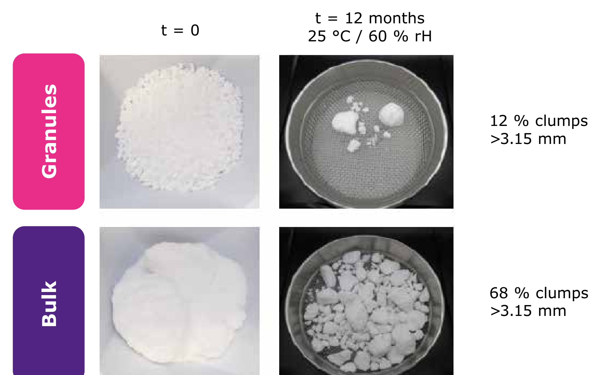
Figure 4: Comparison of caking behavior of bulk and granulated material before and after storage under ambient conditions: example urea.
