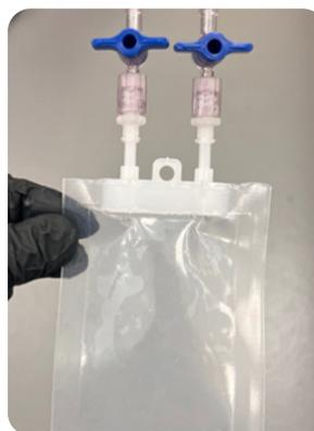
**Figure 1:** Image illustrating the test article PureFlex™ film bag with two ports.
