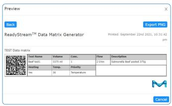
Scan the corresponding data matrix on the ReadyStream® system when prompted using the barcode reader. The information from the data matrix code will be displayed on the dispensing unit of the ReadyStream® system.
