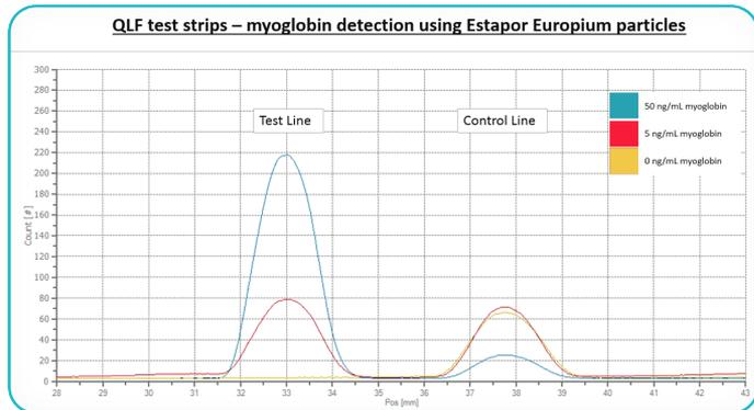
**Fig. 6** Myoglobin detection on lateral flow test strips
