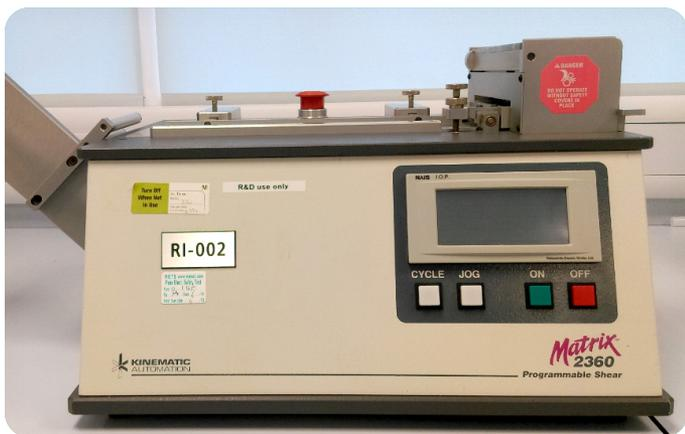
**Fig. 5** Kinematic Matrix™ 2360 Programmable Shears
