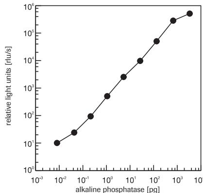
**Fig. 2:** Alkaline phosphatase (intestinal) calibration curve. Serial dilutions of alkaline phosphatase in a volume of 10 µl were applied to a black microtiter plate. The detection was performed with 150 µl substrate reagent according to section 2.1. 10 min after addition of substrate reagent the light signal was measured on a Berthold LB 96 P Luminometer with 1 s integration time.
