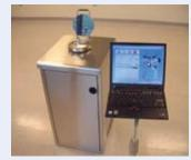
Substrate Size ..... up to 4-in wafers and up to 8-in wafers Substrate Temperature ..... 25–400 °C;  $\pm$ 0.2 °C Precursor Sources ..... 2, heated Deposition Uniformity ..... <1% Footprint ..... 500 × 550 mm Deposition ..... High speed/high aspect ratio Cleanroom Compatibility ..... Class 100
