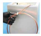
**3.** Connect the grounding cable to a ground point by attaching the clamp to a metal cold water pipe or other earth ground. Consult a qualified electrician if in doubt about the earth ground.
