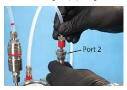
**4.** Make sure the ¼ in. o.d. tubing from reservoir Port 3 is terminated into a fume hood during the degassing procedure.
