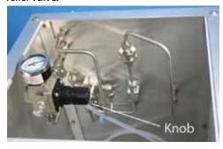
**2.** Check that a vacuum source is connected to Pure Solv Micro and the (pump) exhaust is vented to a fume hood.
