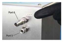
2. Connect a vacuum source to Port 6 (top connection) with <sup>3</sup>/<sub>8</sub> in. i.d. vacuum hose. There is a custom adapter available for connecting multiple Pure Solv™ Micro systems to a single vacuum source. Please contact Sigma-Aldrich Labware for information about these adapters, labware@sial.com.
