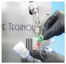
3. Attach a suitably configured collection flask to the 24/40 dispensing joint. A septum-inlet flask, solvent storage flask, or storage/dispensing flask is recommended to enable manipulation of the dry solvent or removal of the flask for use at another location. European joint 24/29 flasks will fit provided there is no constriction in flask neck within 11 mm of the bottom of flask joint. Secure flask with a joint clip.
