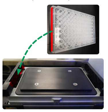
Place the well plate skirt (left edge) up against the flat left side rail of the heated shaker approximately centered (forward/back)
