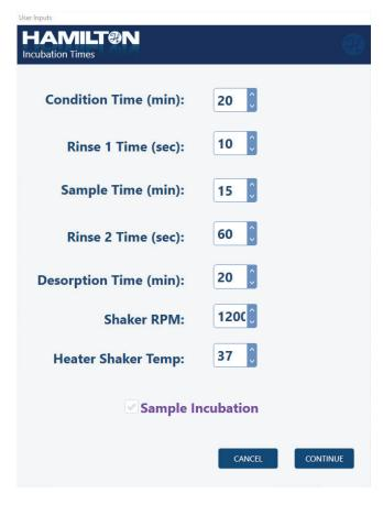
This screen allows for setting the timing, shaker speed, and shaker temperature for processing.
