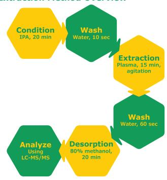
Conditioning—Program the robot to immerse the pin device into the conditioning plate (100% 2-propanol) for 20 minutes without shaking.
