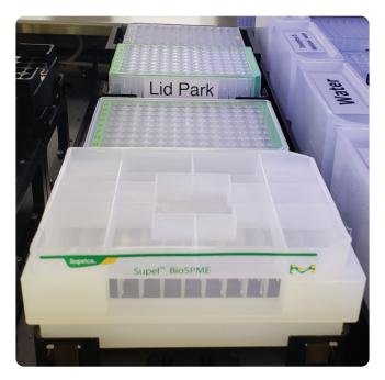
4. Load the Supel™ BioSPME C18 96-Pin Device into the adapter, the adapter should be positioned in place of 96-well plate.
